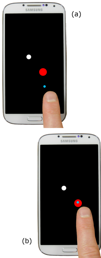
Figure 2. The 2D-Fitts' task has a home location (currently active, red) and a target (currently inactive, white) for each trial. In (a) the user's finger controls the blue Hover Cursor approaching the home location. In (b), the Hover Cursor is in position over the home location. When the user taps, they will select the home location.
