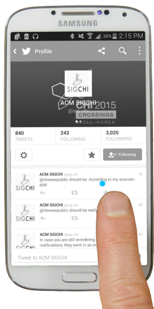
Figure 1. Twitter for Android is an example of an application that has small targets (to reply, retweet or favorite a tweet). Hover Cursor shows the position of the user’s hovering finger as a blue semi-transparent circle that is 2mm in diameter. To reduce occlusion we applied vertical and horizontal offsets.
